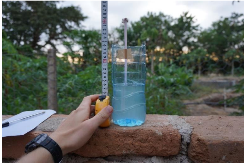
Figure 31: Home-made Barometer – A plastic water bottle the basin of water. A straw, gum, and tape form the chamber in which the liquid can rise and drop with air pressure.
